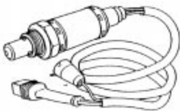
Heated oxygen sensor (HO2S), also called lambda ( \lambda ) sensor.
