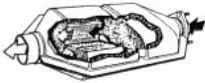
The three-way catalytic converter.
