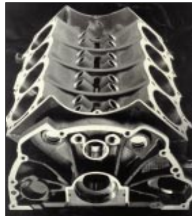
The cylinder block of a V-8 engine
